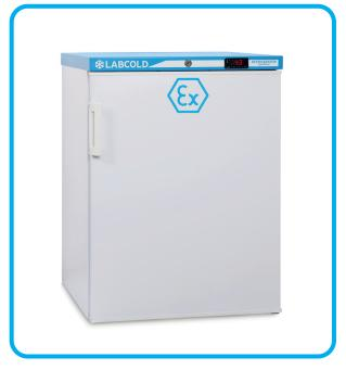
The Labcold ATEX refrigerator range has been designed with an interior which is licensed as a Zone 2 hazardous area under 2014/34/EU (ATEX Directive) in order to store products which are classed in explosion group IIB+H2 and temperature class T6 under 2014/34/EU (ATEX Directive).
