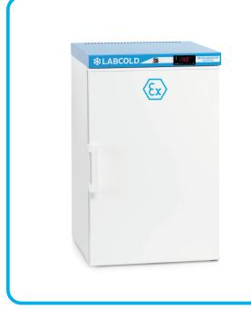
The Labcold ATEX refrigerator range has been designed with an interior which is licensed as a Zone 2 hazardous area under 2014/34/EU (ATEX Directive) in order to store products which are classed in explosion group IIB+H2 and temperature class T6 under 2014/34/EU (ATEX Directive).
