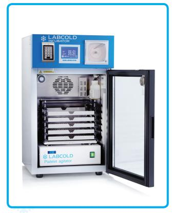
Developed specifically for the safe storage of platelets at the optimum temperature. This Incubator is designed to ensure MHRA compliance.
