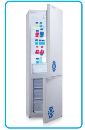
This **Labcold** Sparkfree fridge freezer is engineered to store flammable materials safely with all potential sources of ignition, such as the thermostat removed from inside the compartments of both the fridge and the freezer.
